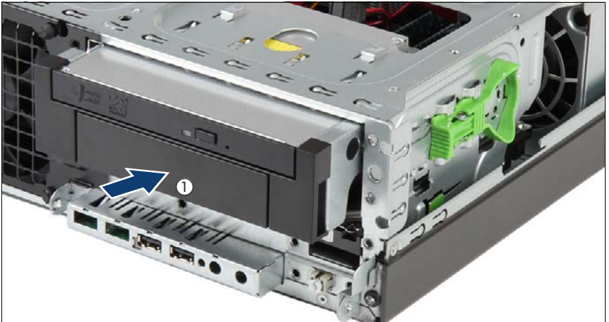
Figure 44: Inserting ODD/HDD bracket in 5.25-inch chassis bay
